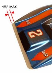
3. **Spoilers and Air Control:** A single, flat plastic spoiler set at any angle may be attached to the rear of the body or under the rear of the body on the vertical portion behind the body. Spoilers may not be attached on top of the body.
